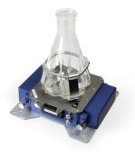
The SFR vario BM offerns non-invasive online monitoring of biomass in shake flask cultures, and additionally measures temperature and rpm. PreSens' optical biomass measurements are based on scattered light detection, so no integrated sensors are necessary. The biomass data can be correlated with parameters like optical density, cell dry weight or cell concentration, so one can get real-time information on e.g. OD600 development.
