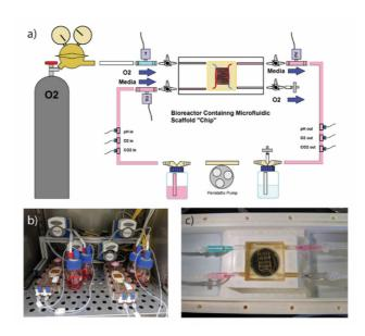
To measure oxygen transfer, they used PreSens' optical oxygen sensors placed directly in the fluid perfusion pathway both at the inlet and outlet of the scaffold. Using this set-up, they have shown that their lung-on-a-chip model achieves similar rates of oxygen transfer, when normalized by gas exchange surface area, as that seen in commercial oxygenators.
