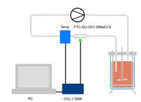
A fed-batch-process with Horizon's glutamine synthetase knockout CHO cell line was carried out in an autoclavable 10L benchtop bioreactor. For online culture monitoring PreSens' novel pCO2 measurement system - with the sensing element installed within a bypass - was applied. The online measurements were in good agreement with gold standard Bioprofiler's offline pCO2 measurements.
